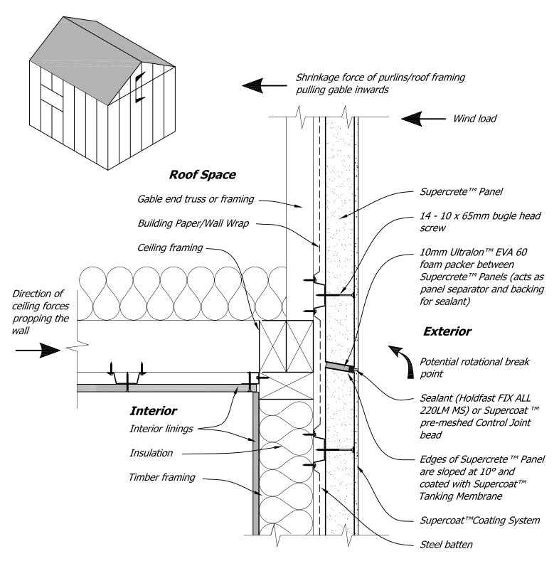
**NOTE:** This detail is required where a ceiling intersects the wall, except where the height from ceiling to gable apex is greater than 2000mm or where a mid floor intersects, use Details SPC 3-6, page 31, or SPC 3-7, page 32
